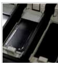
Automated application of oil for sealing
