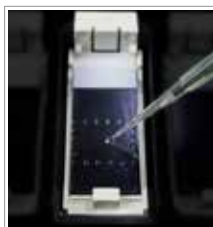
Manual dispensing of micro-reagents (proteinase, probe and DAPI)
