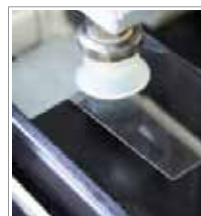
Automated mounting and final coverslip after DAPI
